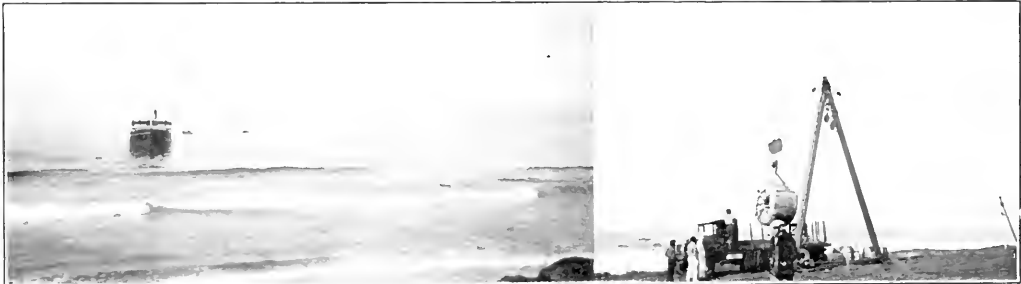
The Richfield tanker Tamiabua, now undergoing repairs at the Union Plant of the Bethlehem Shipbuilding Corporation, after stranding near Pescadero Point. Due to the rough weather encountered it was necessary to rig a high line from the bow of the vessel to the shore a distance of 900 feet. The illustration shows the tanker in the surf with the lines and the shear legs on the shore end.
